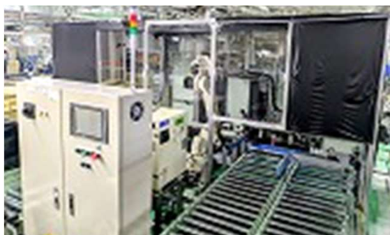
Cameras automatically detect paint scratches, unevenness, and paint pools on parts
